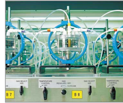
Static load method : proof ring type
