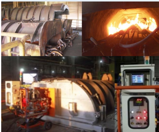
1 — [Before] Direct heat drying 2 — [Improved] Hot-air drying
