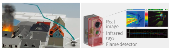
Unmanned flexible fire apparatus (boom length: 60 m)
