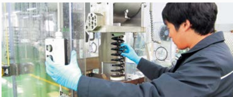
POSCO developed a high tension coiled spring through joint research with its partner DAWONKANGUP. An employee at DAWONKANGUP is testing the corrosion resistance of coil springs.
