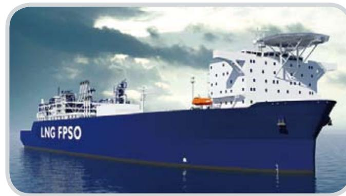
FPSO (Floating Production Storage and Offloading)
